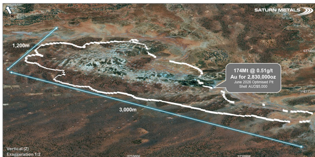
Plate 1 – Topographic aerial view of Apollo Hill, June 2026 nominal constraining pit shell 1 boundary and drill pads (looking North); Satellite photography taken on 9 June 2023. 1:2 vertical (Z) exaggeration applied to pronounce outcropping hills and topography.
