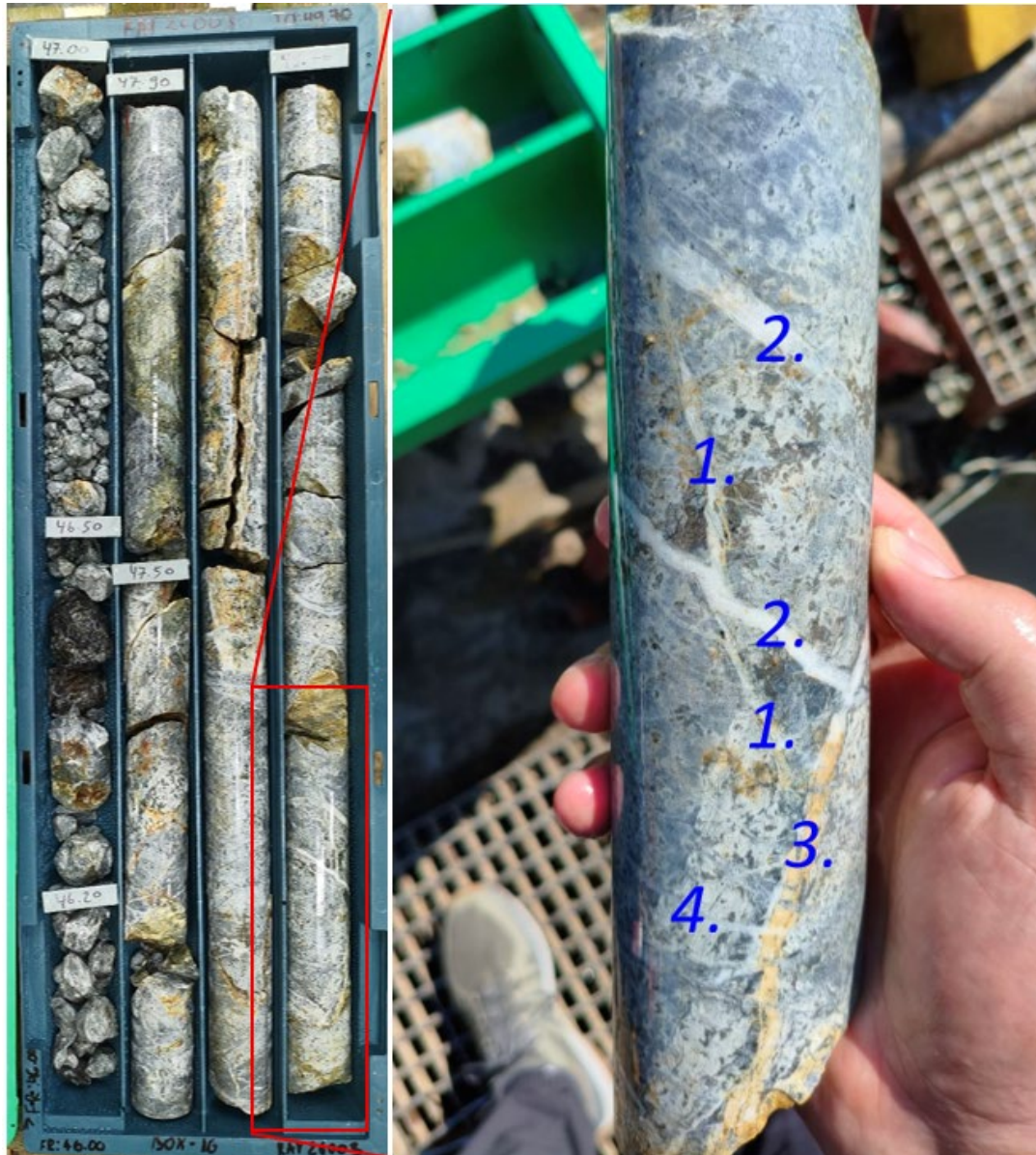
Figure 3. Diamond drill core from 49.3 m RAV26003 showing stockwork veinlets cross-cutting highly silicified breccia containing disseminated sulphide.
