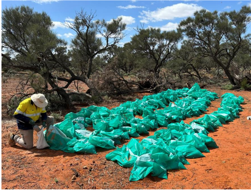
Figure 3: Sheoak Prospect - Collecting Metallurgical Test Work Material from AUV RC Drill Samples
