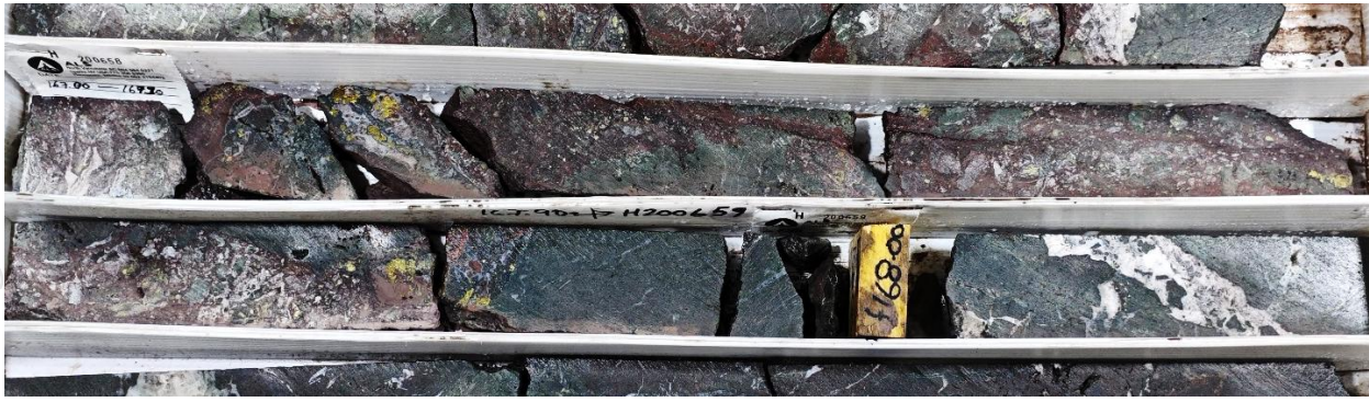
Figure 5. Section of cut core showing a complex breccia zone with hematite (brown), quartz (white) and the copper sulphide mineral chalcopyrite (yellow). Peak assay grades from this zone included 0.9m at 467g/t Ag, 0.6g/t Au, 1.4% Cu, 1.4% Pb & 2.1% Zn from 169m down hole.
