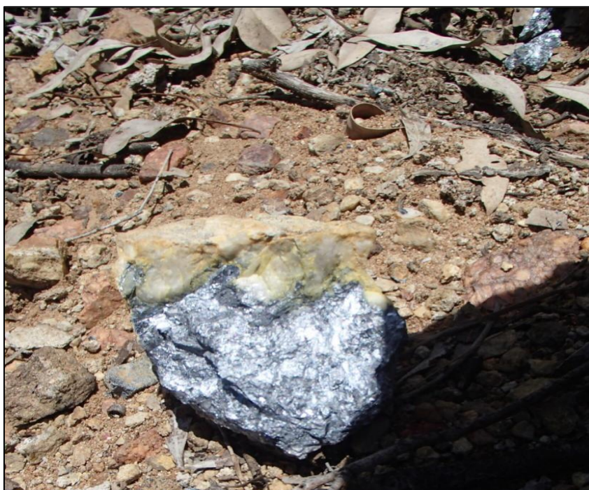
Figure 5: Banshee mine waste dump material observed (unsampled) by Dart Mining in January 2025 showing antimony mineral (70% stibnite*) with encasing vein quartz.*
