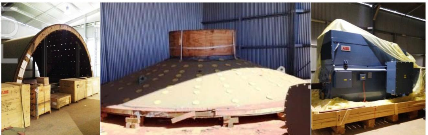
Figure 1. New SAG mill components and drive motors
