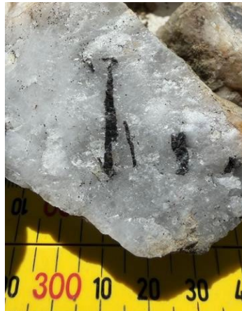
Figure 2. Sample no 105496. Vein no 3 (4.32% W). Close-up of acicular wolframite to 3cms in Type 2 glassy vein quartz
