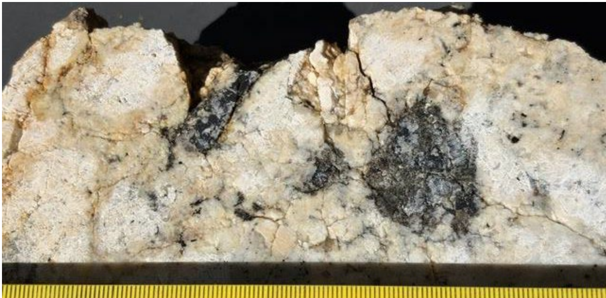
Figure 3 Sample no 105498 (3.04% W). Vein no 3. Field of view approximately 22cm. Coarse patches of biotite and wolframite within a coarse weakly brecciated pegmatitic granite.
