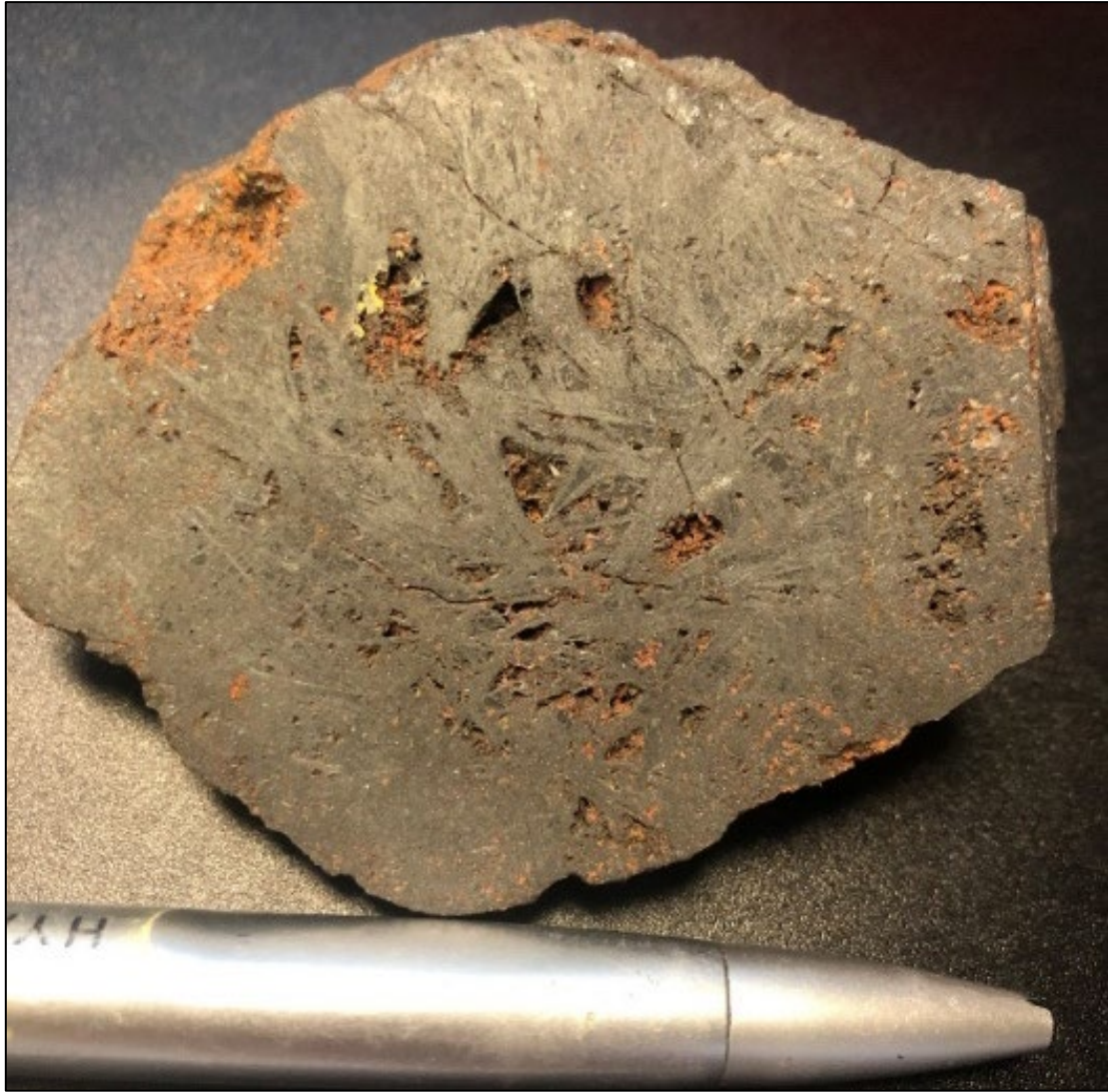
Figure 11: Burringa East rock float sample of bladed magnetite 2.5g/t Au, 0.4% Cu, 112ppm Mo, 26ppm Bi, 3ppm Te (17R1043). See Figure 14 for location.
