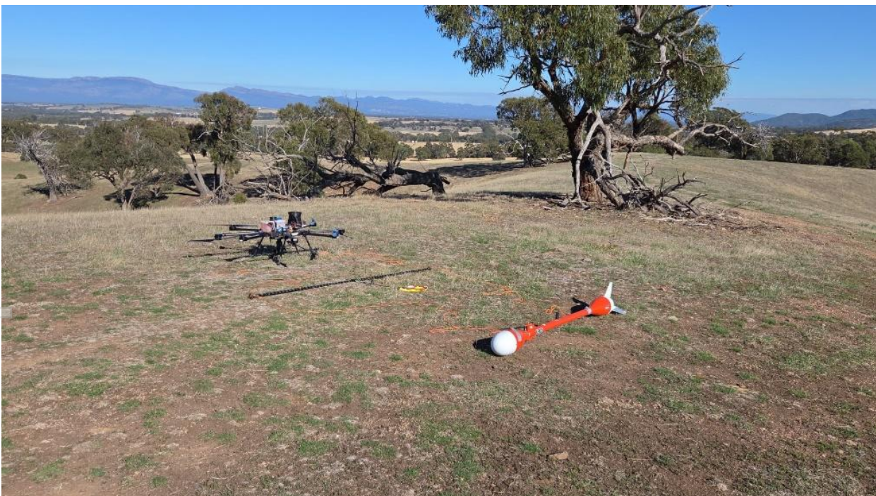
Figure 3: Preparation of drone and magnetometer on the ground prior to commencement of survey
