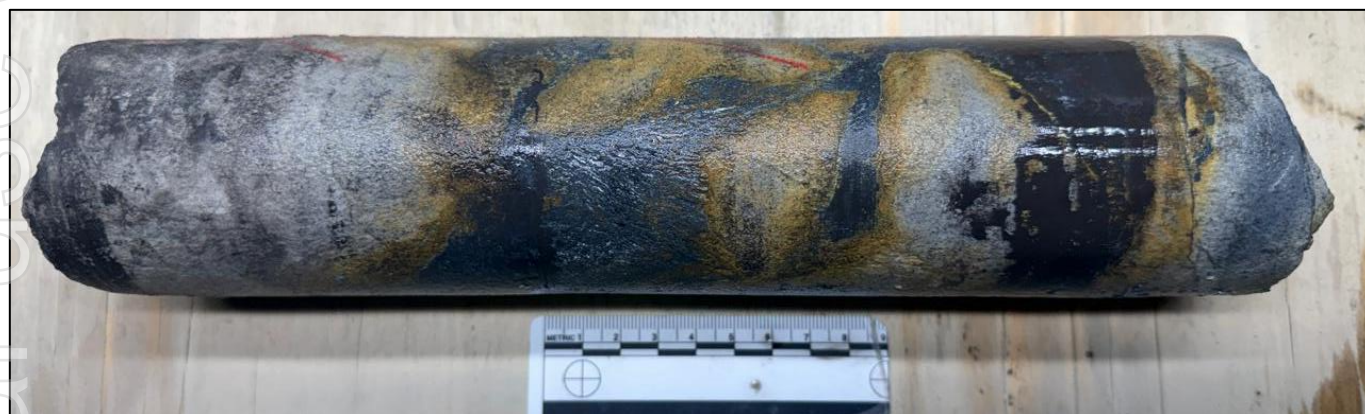
Figure 4: ACP26DD026 core sample 1103384 from the high-grade pod interval, returning 42.10% Sb. Wet core photograph showing dark steel-grey to black massive to semi-massive acicular stibnite replacing the sandy Salt and Pepper tuff and infilling fractures and pore spaces. Grey-beige altered tuff remnants, orange-brown oxide halos and minor veinlet textures are visible along the margins, supporting a carbonate dissolution and pore-space replacement style of mineralisation.
