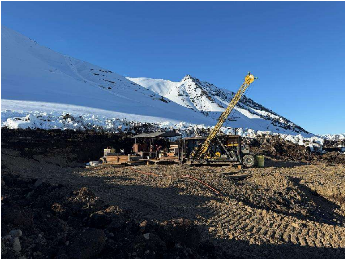
Figure 5. Diamond drill rig commences 10,000m oriented diamond core at Caribou Dome (CD26-01) testing an IP anomaly.
