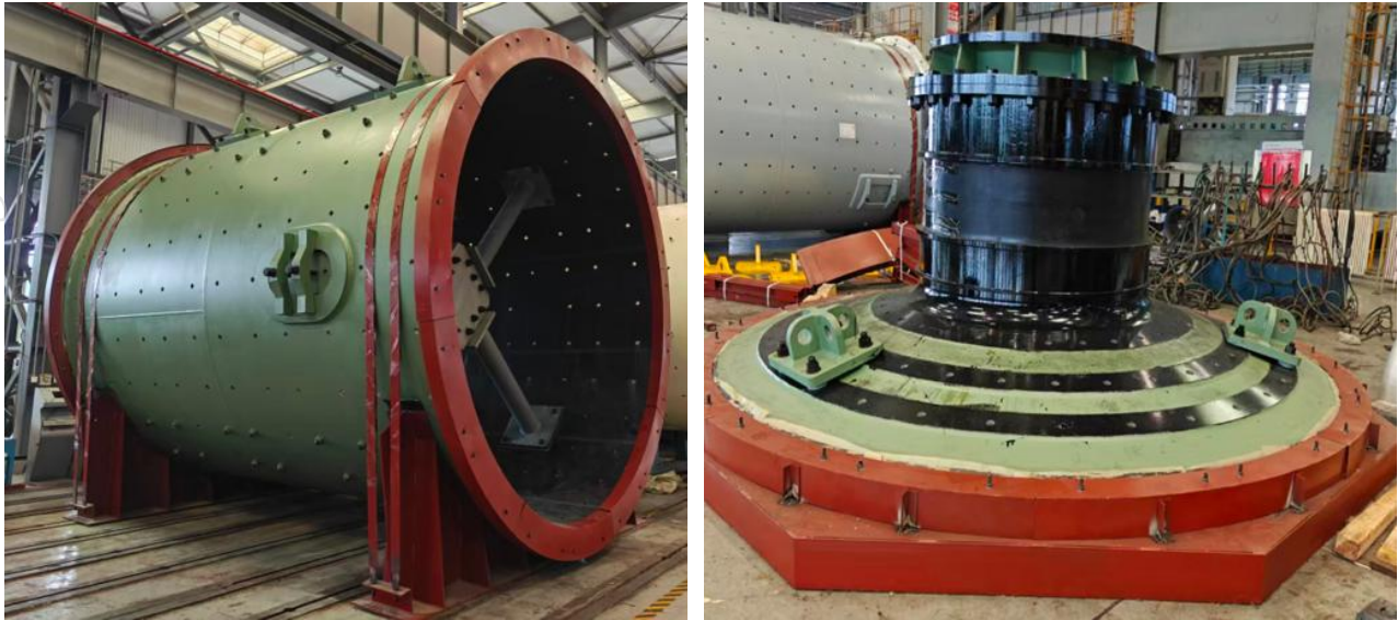
Figure 2: Ball mill shell (left) and head (right)
