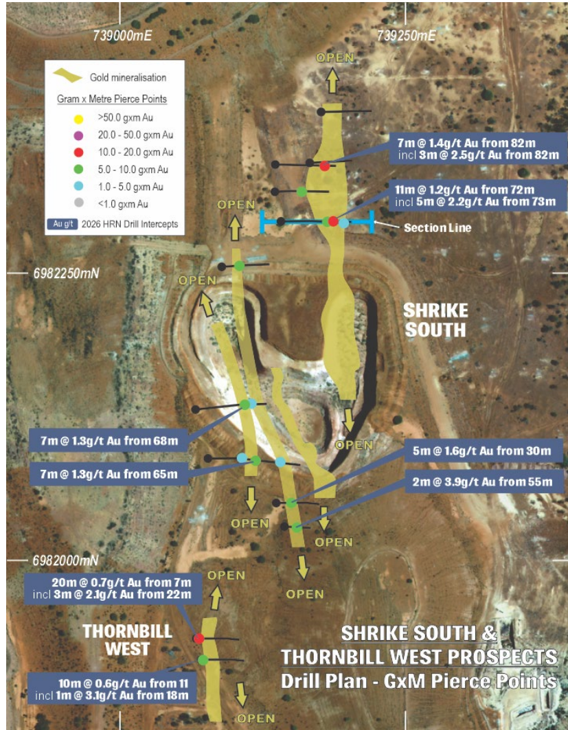
Figure 7: Shrike South & Thornbill West drill hole plan showing recent drill intercepts (>6 GxM) & gram x metre pierce points over satellite image.
