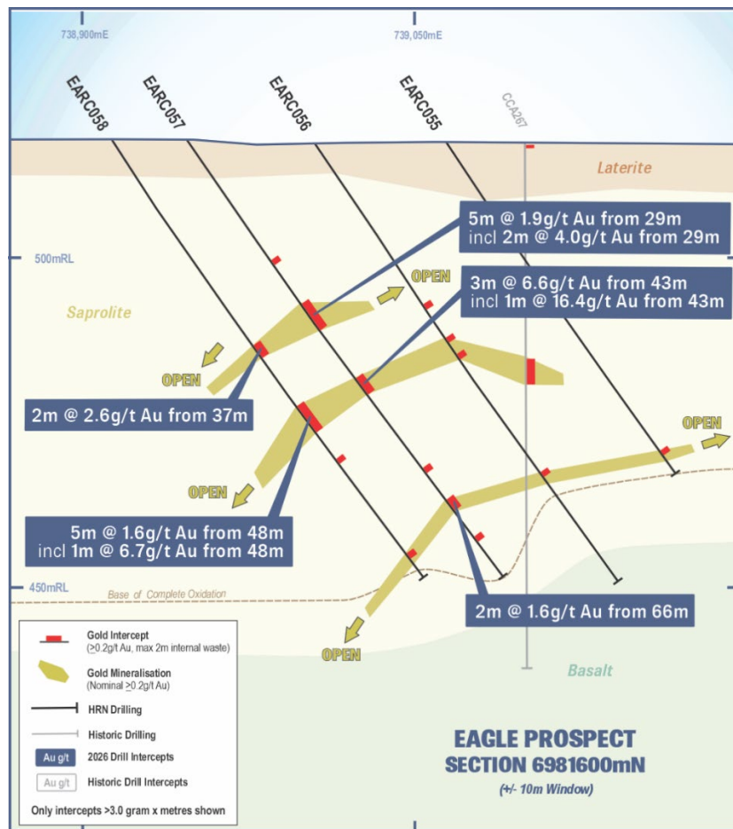
Figure 5: Eagle cross section showing interpreted mineralised zones and significant 2026 RC intercepts (>3 GxM).
