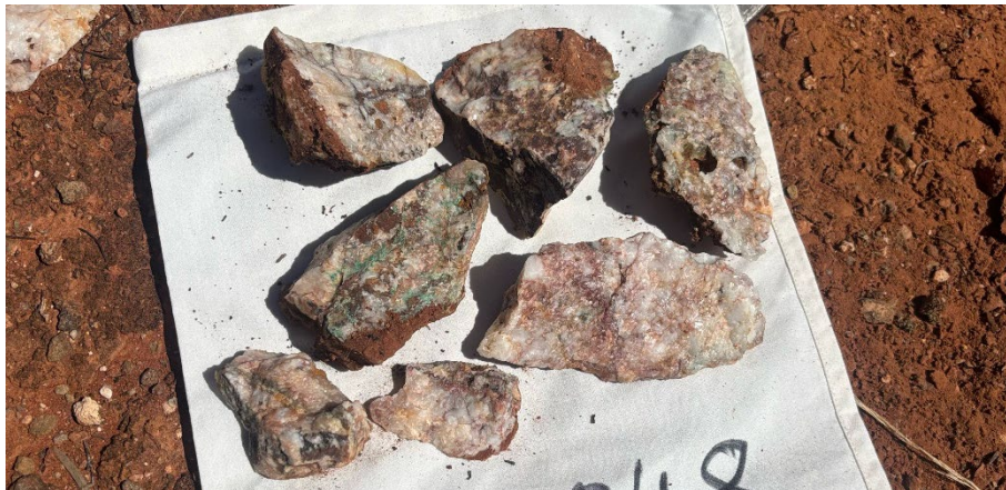
Figure 2: Rock chip samples of vuggy quartz-k-feldspar-carbonate and possible malachite that returned 11.78 g/t Au, 19.5 g/t Ag and 0.18% Cu (SMZS048)
