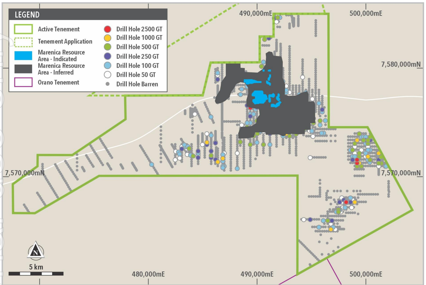
Figure 2 Resource Outline with Grade Thickness (GT) Collars Located Outside of the MRE
