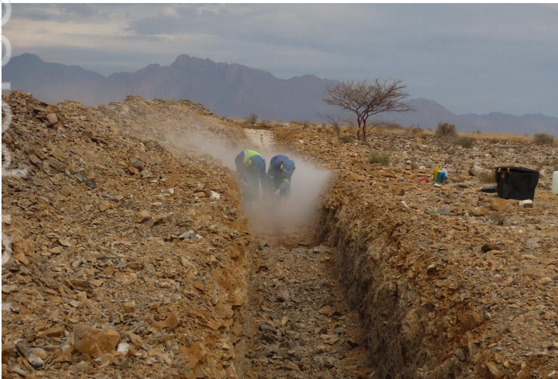
Image 2: Example of the trenching completed at the K9 Target. Trenches are dug using a mechanised excavator to the point of refusal. The trenches are then cleaned manually and mapped by a geologist to document the exposed geology across the width of the pegmatite target and document the host lithology. Visual indicator marks are made across the pegmatite for channel sampling to be completed using a rock saw and hand chisel to remove the sample for bagging and sample preparation. Channel sampling is completed using a rock saw and hand chisel to remove the sample for bagging and sample preparation.
