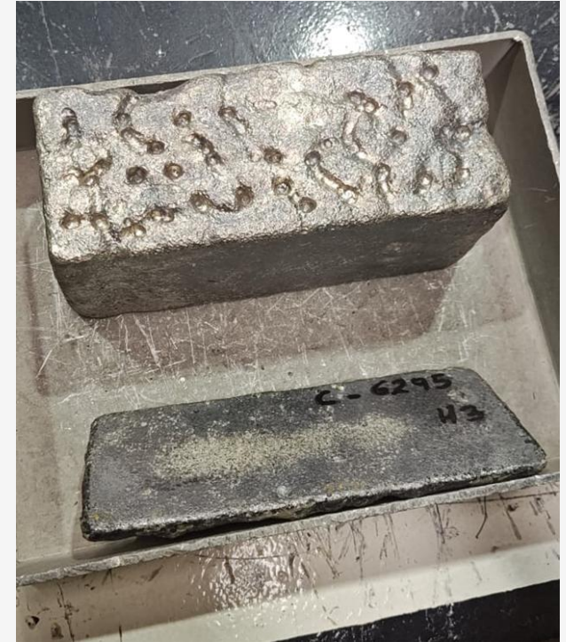
Photo showing first Hualilan Dore Bar with approximately 500 gold ounces and 6,000 silver ounces
