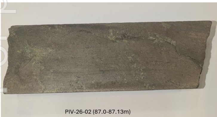
Figure 3: Close up of intense Cu-Ni-PGM mineralisation, rich in chalcopyrite and pyrrhotite
