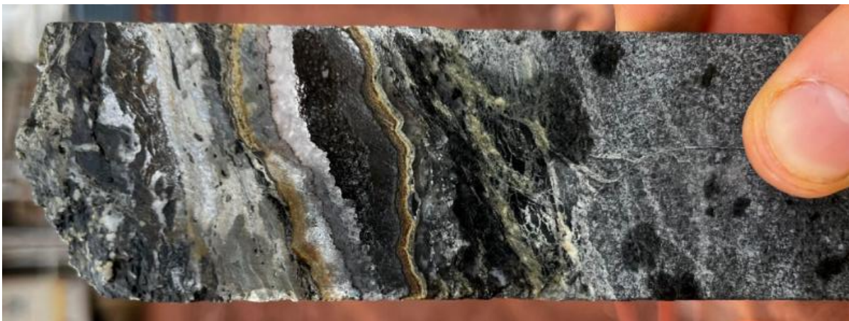
Figure 4. In SWDD009 Hydrothermal vein along contact between mineralised ultramafic unit and dolerite dyke. At 68.4m grading 17.1 g/t PGE3.
