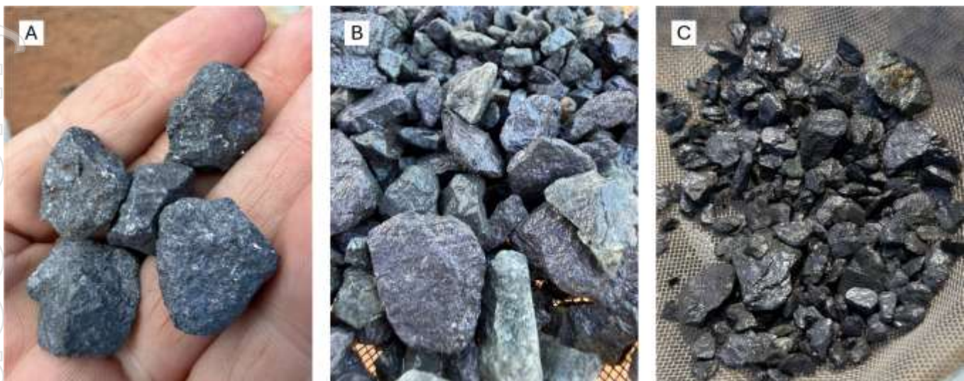
Figure 2 – Examples of galena and sphalerite mineralisation in current drill holes (A) Percussion chips of massive galena mineralisation from BTPRC017 (49 – 50m); (B) Percussion chip samples with strong galena-sphalerite mineralisation estimated at 15% galena and 20% sphalerite 5 in chlorite-altered sediments from BTPRC017 (49 – 50m); (C) Percussion chip samples with strong galena-sphalerite mineralisation estimated at 15% galena and 25% sphalerite 5 in chlorite-altered sediments from BTPRC018 (27 – 28m).
