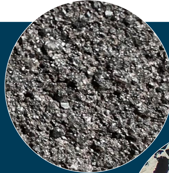
Sub-euhedral magnetite ranging in size from 0.1mm – 5mm
