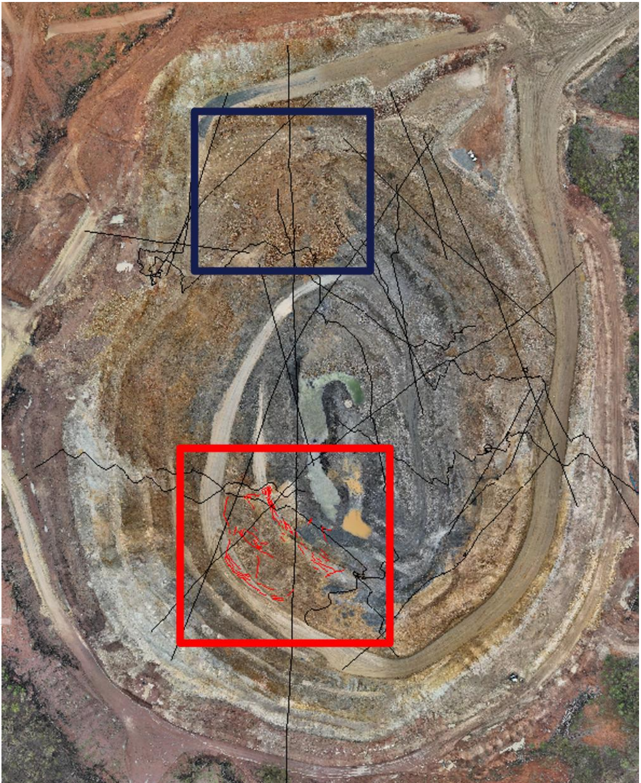
Figure 3: Pearse South Open Pit – Southwest area (red box) shows the area of the new geotechnical incident. Northern area (blue box) shows the area of previous geotechnical incident.
