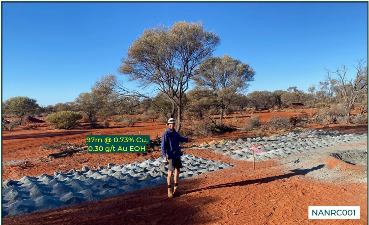
Photo 1. Typical RC drill samples (NANRC001) 3 at Nanadie. Note the limited oxidation profile below shallow sandy soils.
