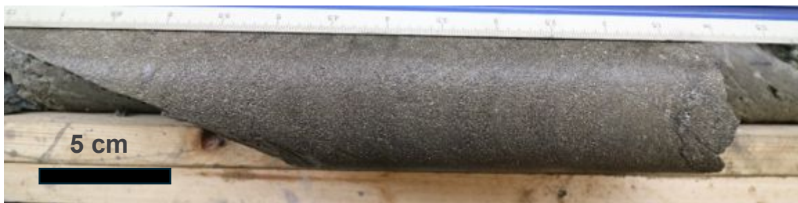
Figure 4: Example of massive sulfide from the Fuego prospect (K26-571, 61.8-62.0m downhole). The interval from 61.0 to 62.0m returned assays of 126g/t Ag, 5.5% Zn, 0.9g/t Au, 0.1% Cu, 3.8% Pb.
