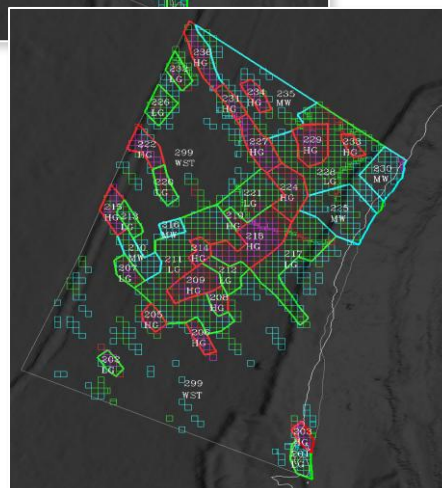
Q3 SMU constrained 0.5 g/t high-grade dig block design
