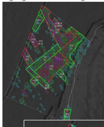
H1 unconstrained 0.5 g/t high-grade block design
