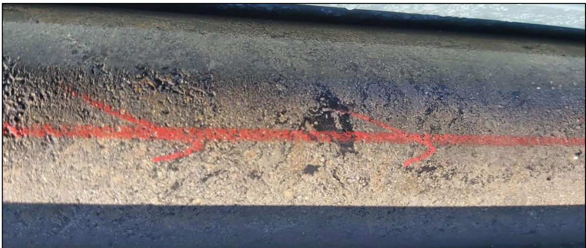
Figure 6: 26DDBR004 massive pyrite (bronze) and sphalerite (brown) 195.0 - 195.2m, grading 3.4g/t Au and 8.4% Pb+Zn over the 1m interval.
