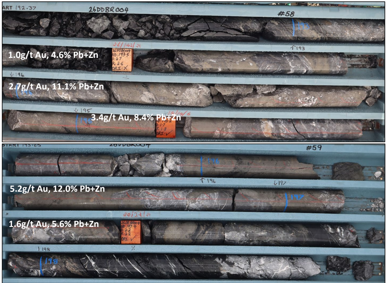
Figure 5: 26DDBR004 massive sulfide zone (brown), dominantly sphalerite and pyrite from 193m to 197.1m grading 5.1m at 2.7g/t Au & 8.3% Pb+Zn.
