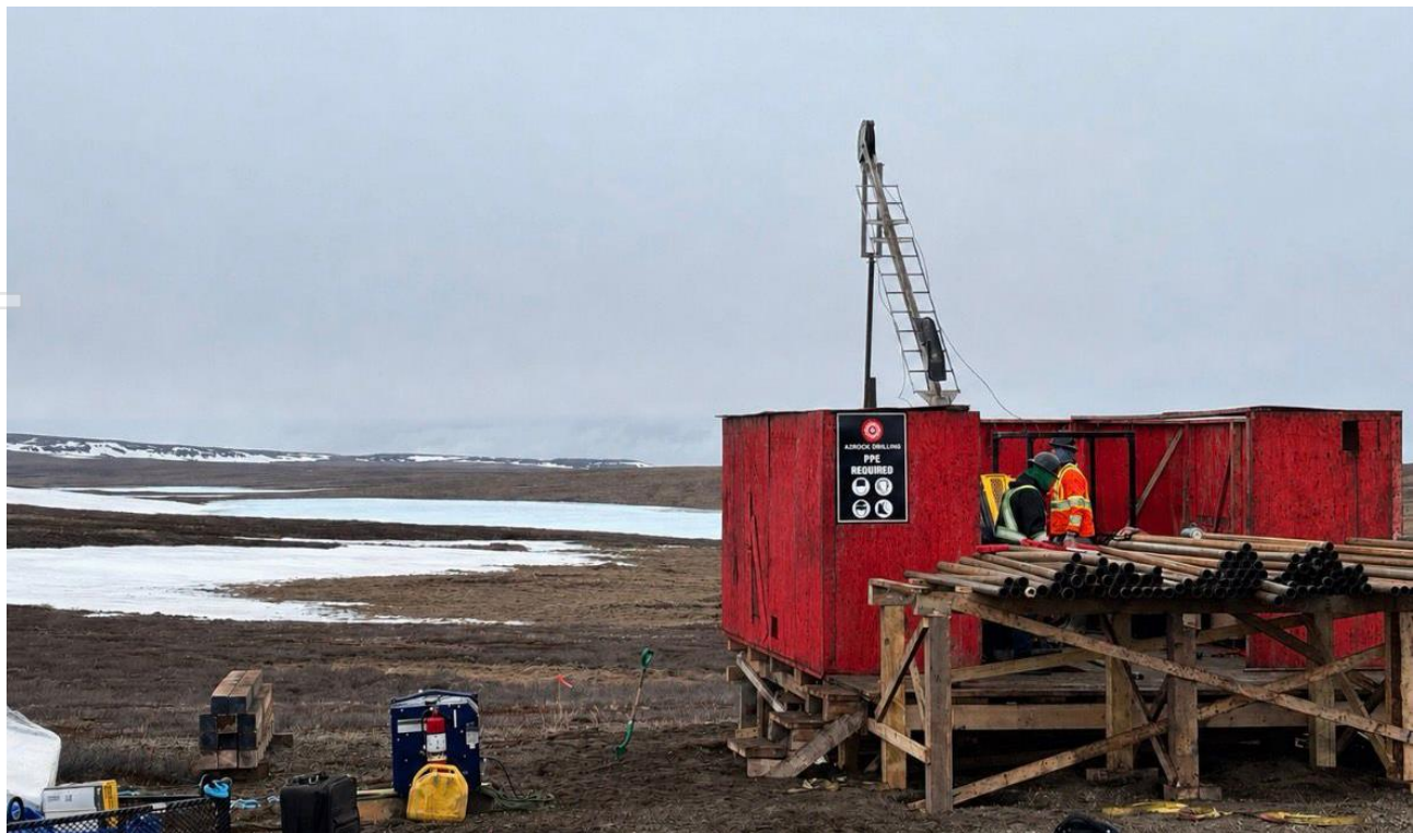
Figure 4 - Photograph of diamond drilling rig positioned over SED26001.
