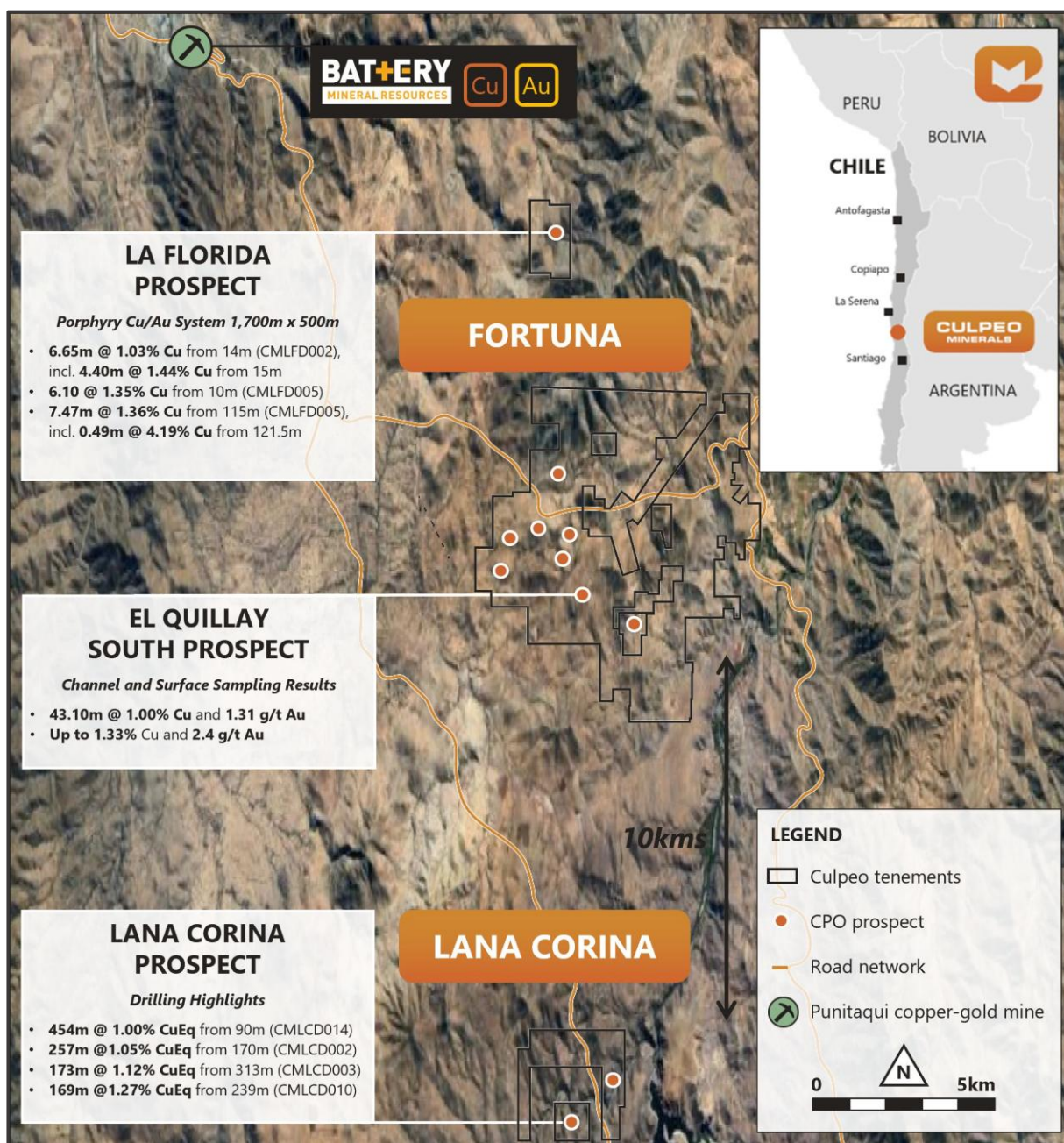
Figure 1: Location of La Florida and El Quillay Prospects within the Fortuna Project 1,2,3,4,5,6,7,8,9,10,11,12 (N.B. see Appendix B for references outlining historic result details)
