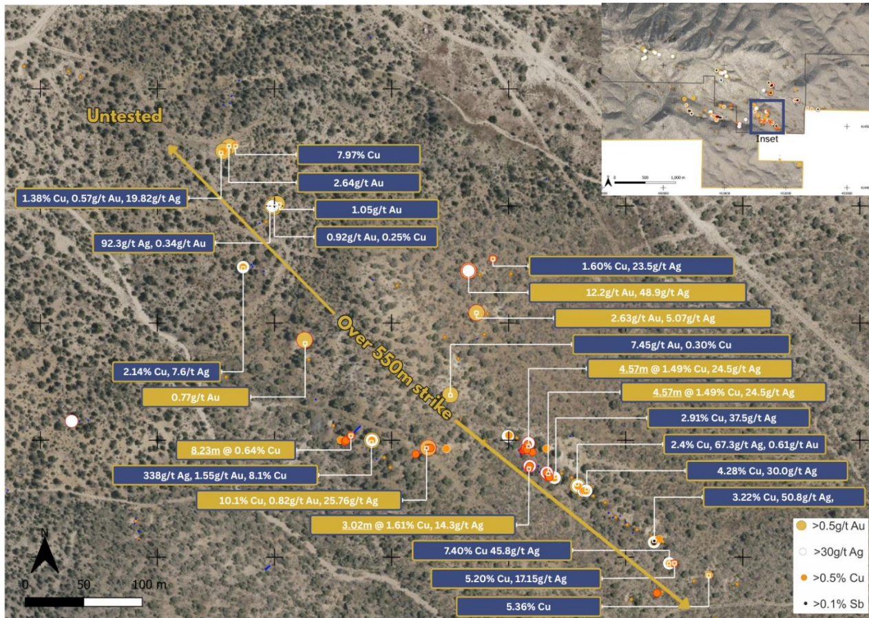
Figure 3: Silver- and copper-rich trend at Blue Dick with new results (gold) alongside previously reported results (blue)
