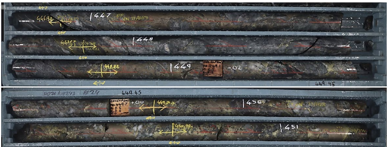
Figure 2: DD26KP1243 – Zone 2, 4.7m intersection of Hillsborough Deeps from approximately 447m downhole, comprising quartz sulphide veining and massive sulphide. The sulphide mineralisation observed has relative abundance of pyrrhotite (25%), chalcopyrite (10%), and pyrite (<5%).
