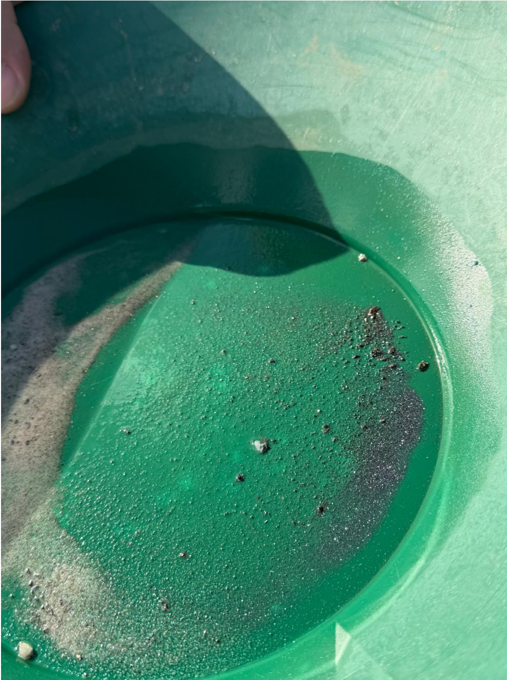
Figure 2: Panned sulphide tail including sphalerite, tetrahedrite and galena ( \pm native silver) from approximately 400 grams of dump sample material; Keystone Project.
