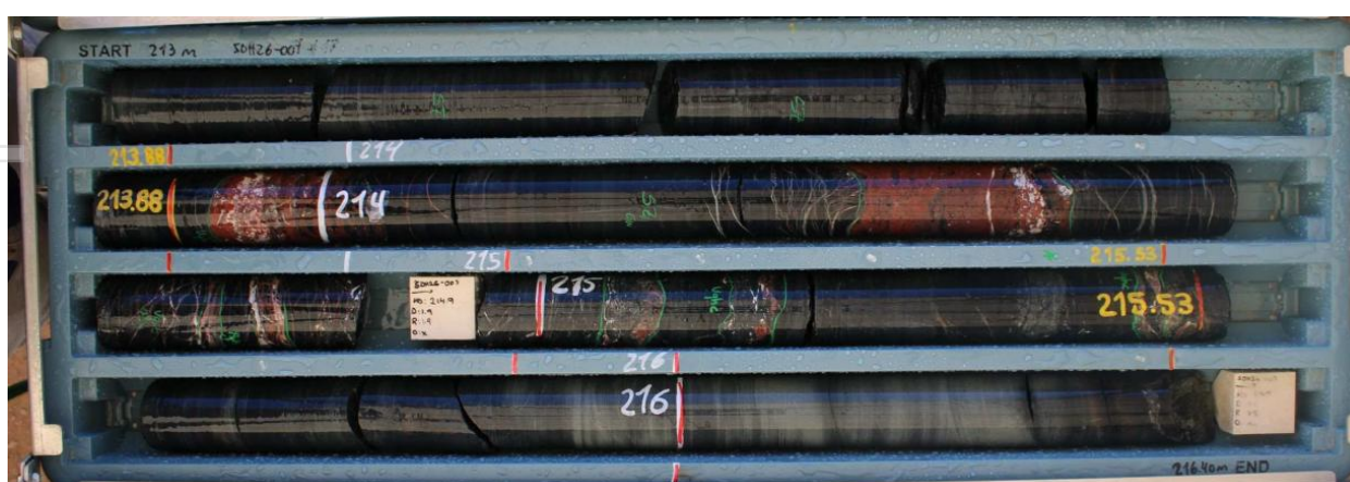
Plate 1 - SDH26-007 Hematite alteration associated with Link Style mineralisation (6.0m @ 5.16 g/t Au from 209.6m)
