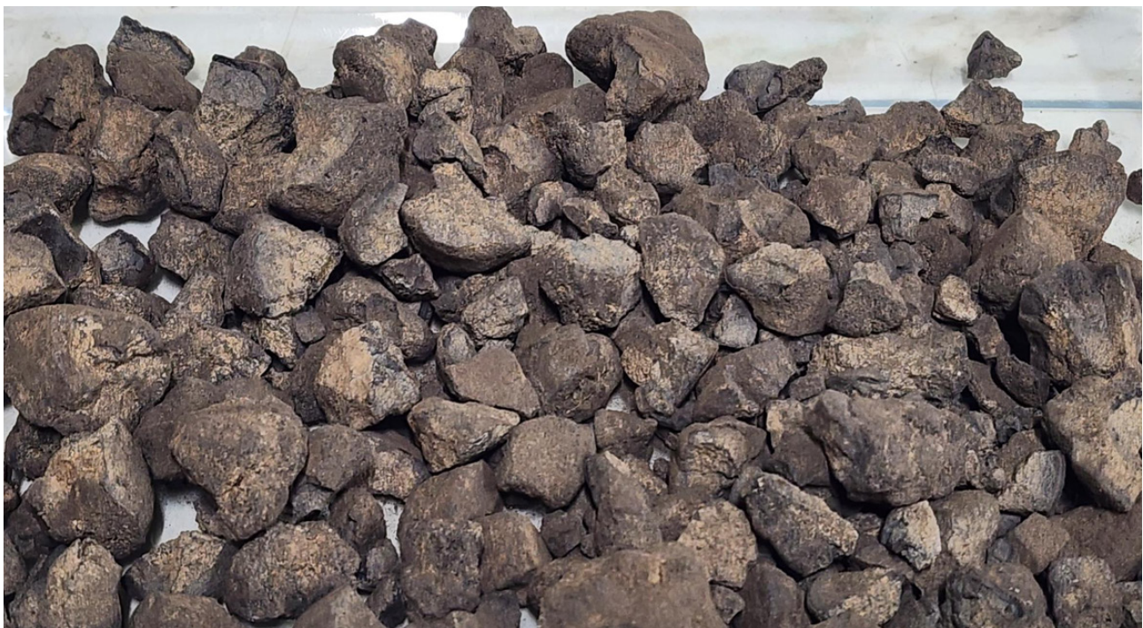
Figure 4 - Samples of polymetallic nodules from the CCZ at the Broken Hill Technology Centre.
