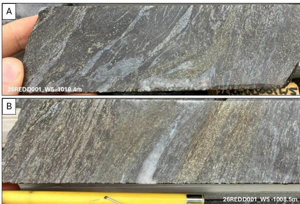
Figure 2: Examples of high-grade gold mineralisation at Triton from 26REDD001_W5; (A) depth 1010.4m returning 28.30g/t Au, (B) depth 1008.5m returning 3.04g/t Au.
