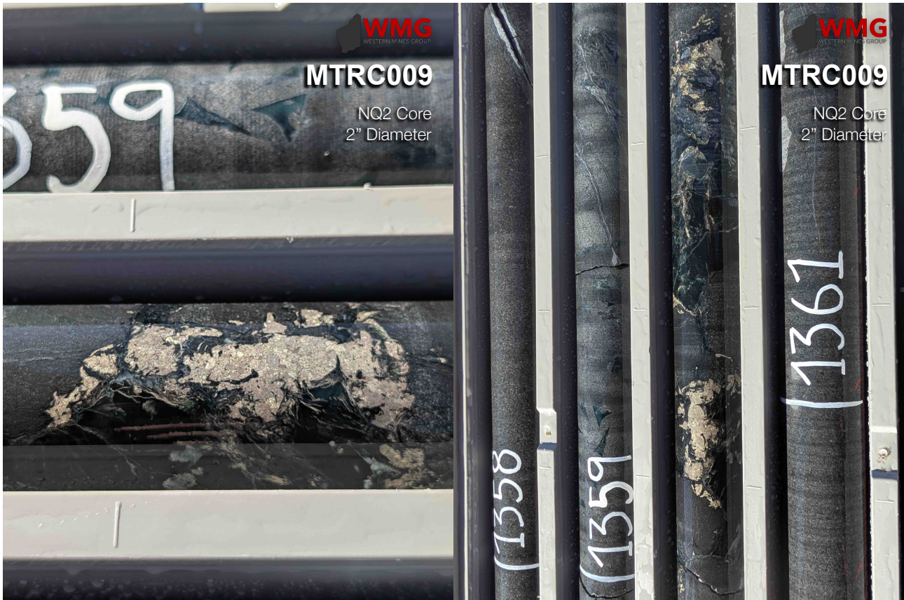
Figure 4: Photos showing examples of sulphide segregations in hole MTRC009 (EIS9) Note: core is NQ2 being 2 inches or 50mm diameter
