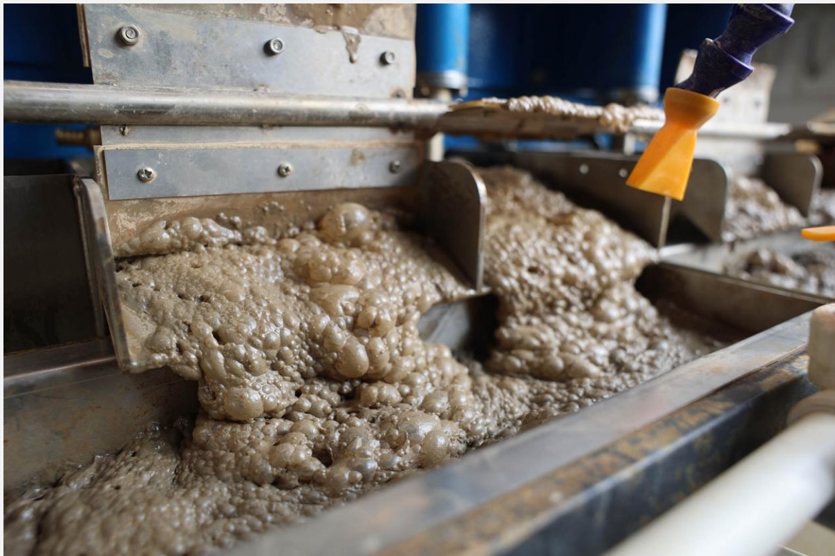
Figure 4. Heavy rare earth enriched froth sourced from clay ore at North Stanmore.
