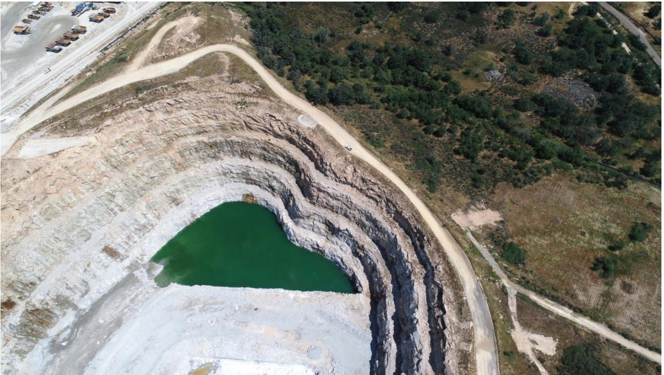
Figure 1: Northern In-Pit Sump
