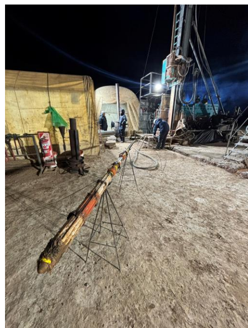
Figure 4. Zelandez Gamma tool being prepared Table 1,2 Table of Zones with Total Porosity and Specific Yield and Assay.
