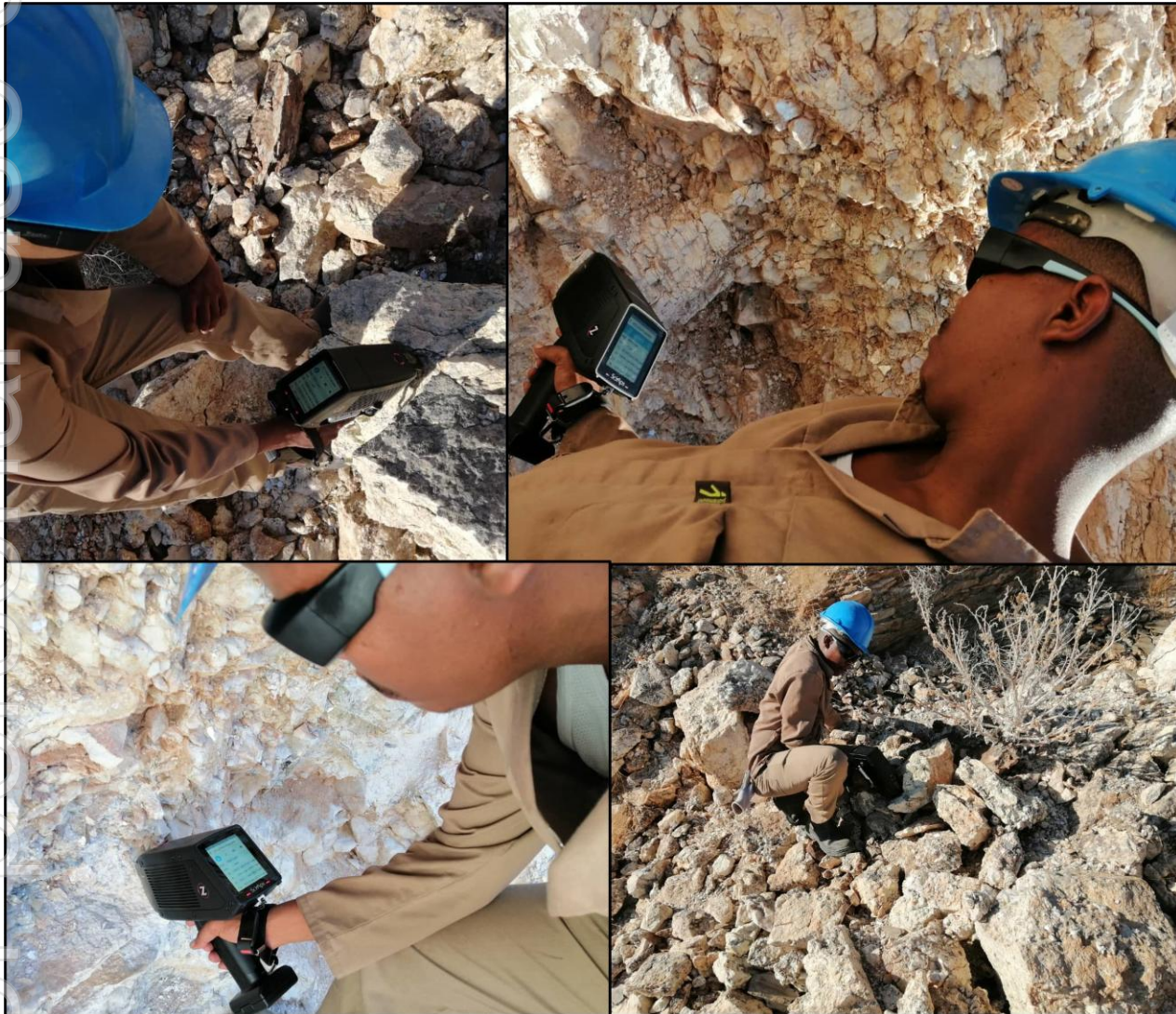
Figure 7: Handheld LIBS (Laser-Induced Breakdown Spectroscopy) instrument used in the field. Here, the team assess the potential of our pegmatite targets using the LIBS to analyse for light elements (Li, Be, Mg and B).
