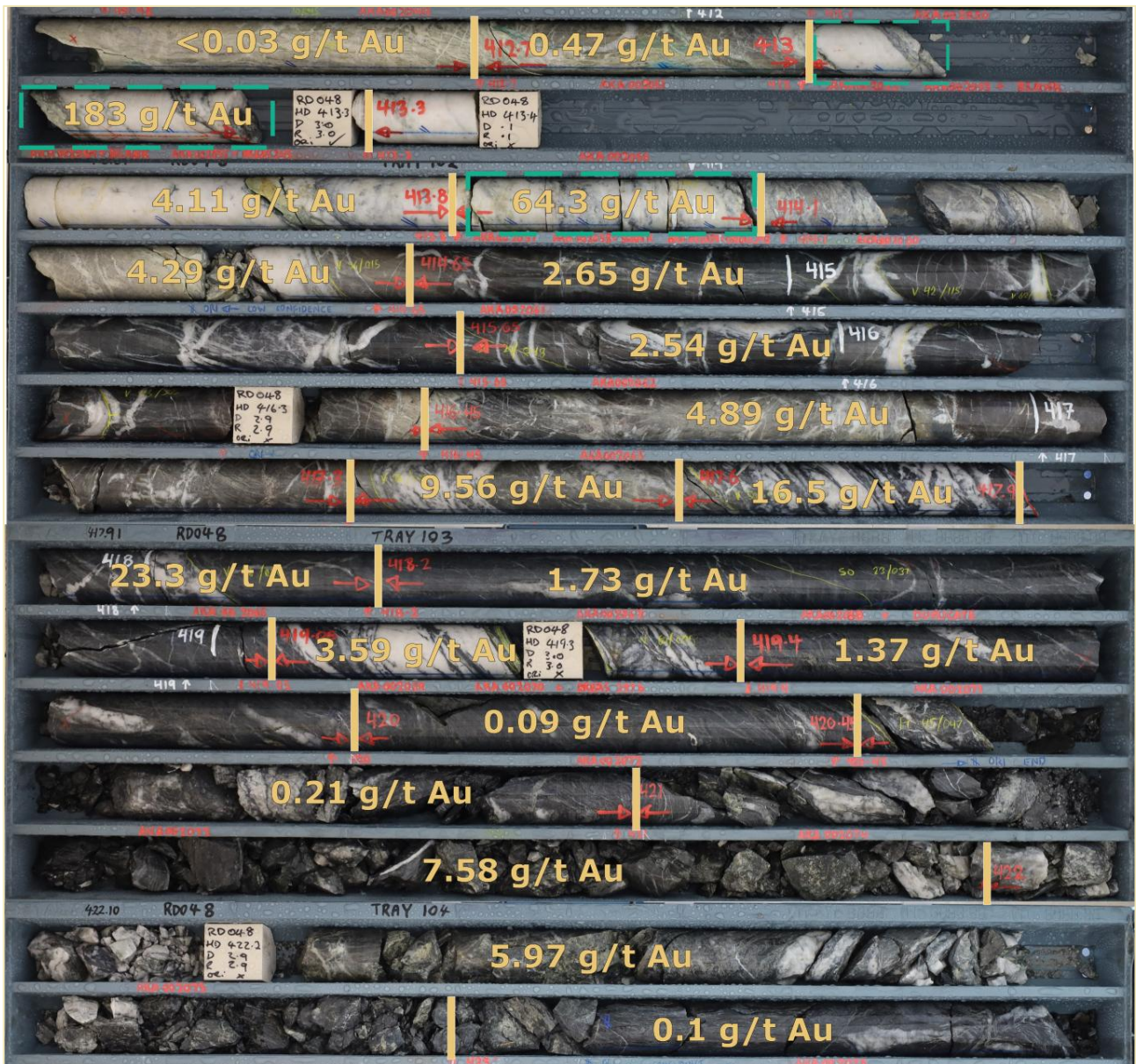
Figure 3: Example of the quartz veining and gold mineralisation contained within the Resolution Lode at the Irvine Gold Project. RD048 intercept 10m @ 12.1g/t Au from 413m as reported on 15 Oct 2025 in ASX Release AKA – Highest Assay Since Discovery.
