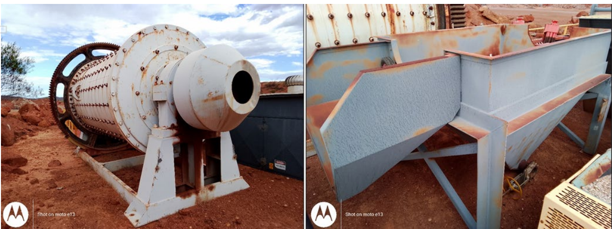
Figure 12: Ball Mill and discharge chute
