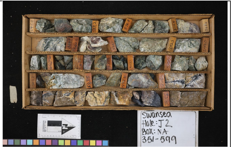
Figure 6: Drill core (split for sampling) from Swansea.
