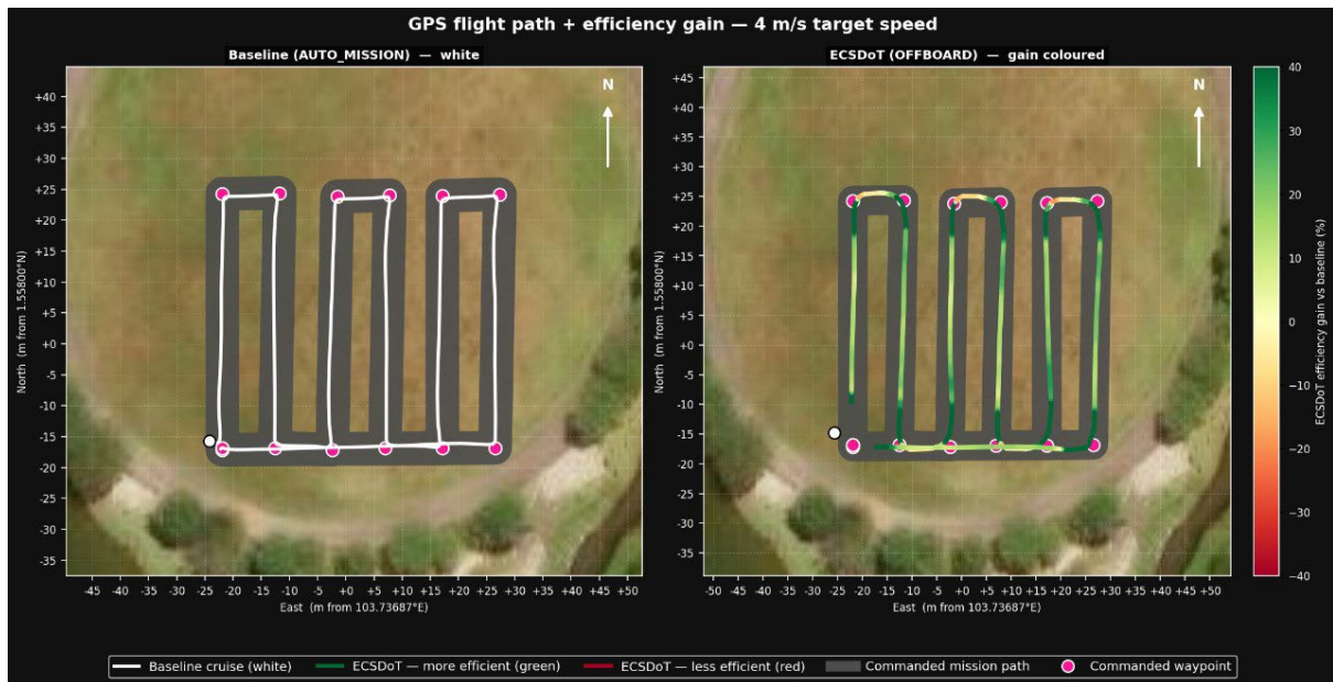
Figure 5: GPS Flight Path Efficiency Overlay at 4 m/s - Baseline (White, Left) vs ECS-DoT Efficiency Gain (Colour-Coded, Right)
