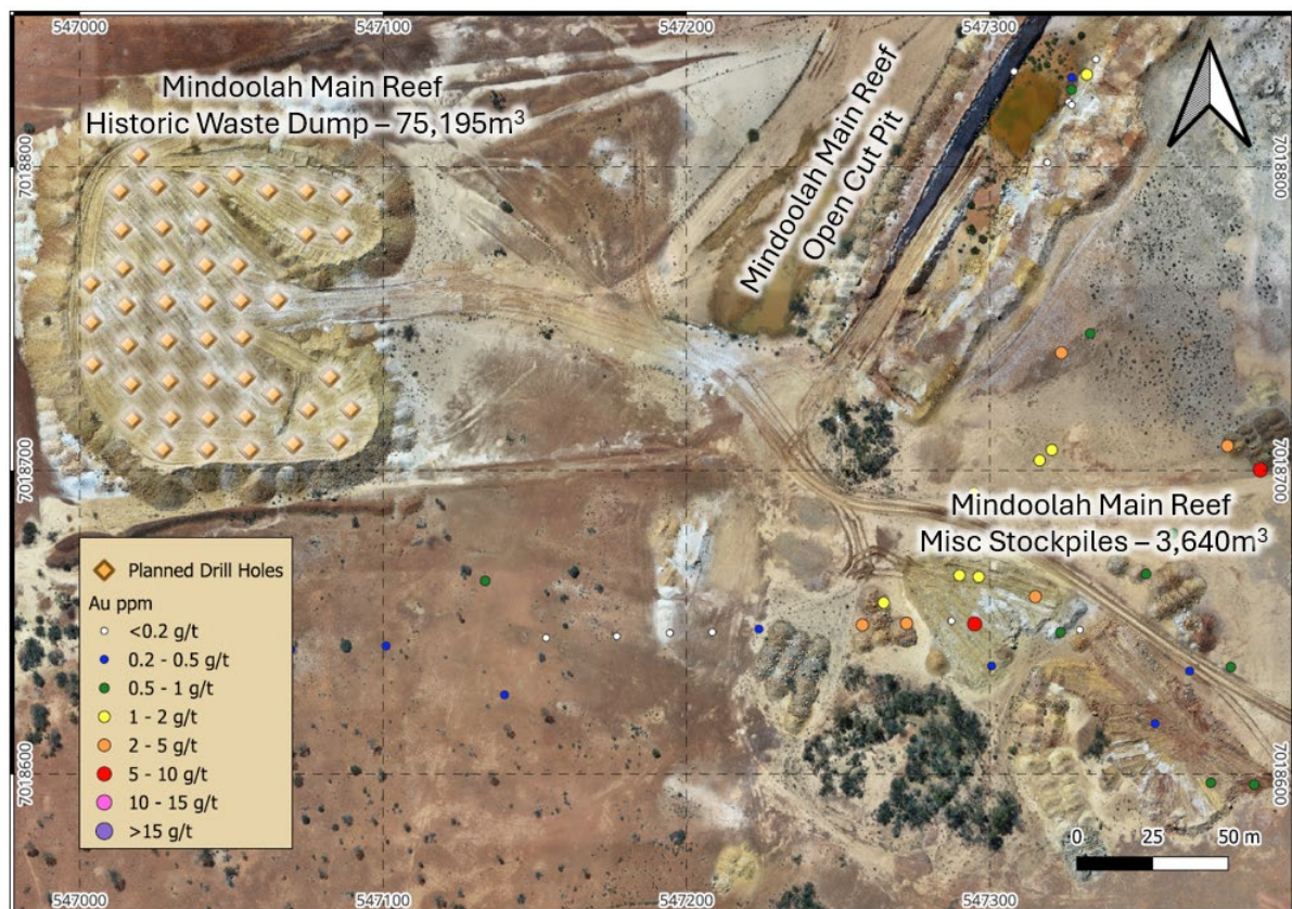
Figure 2. Mindoolah Main Reef Waste Dump Drill Program locations with Historic Rock Chip Grab Samples as coloured dots in surrounding areas (Appendix 1: Table 2).
