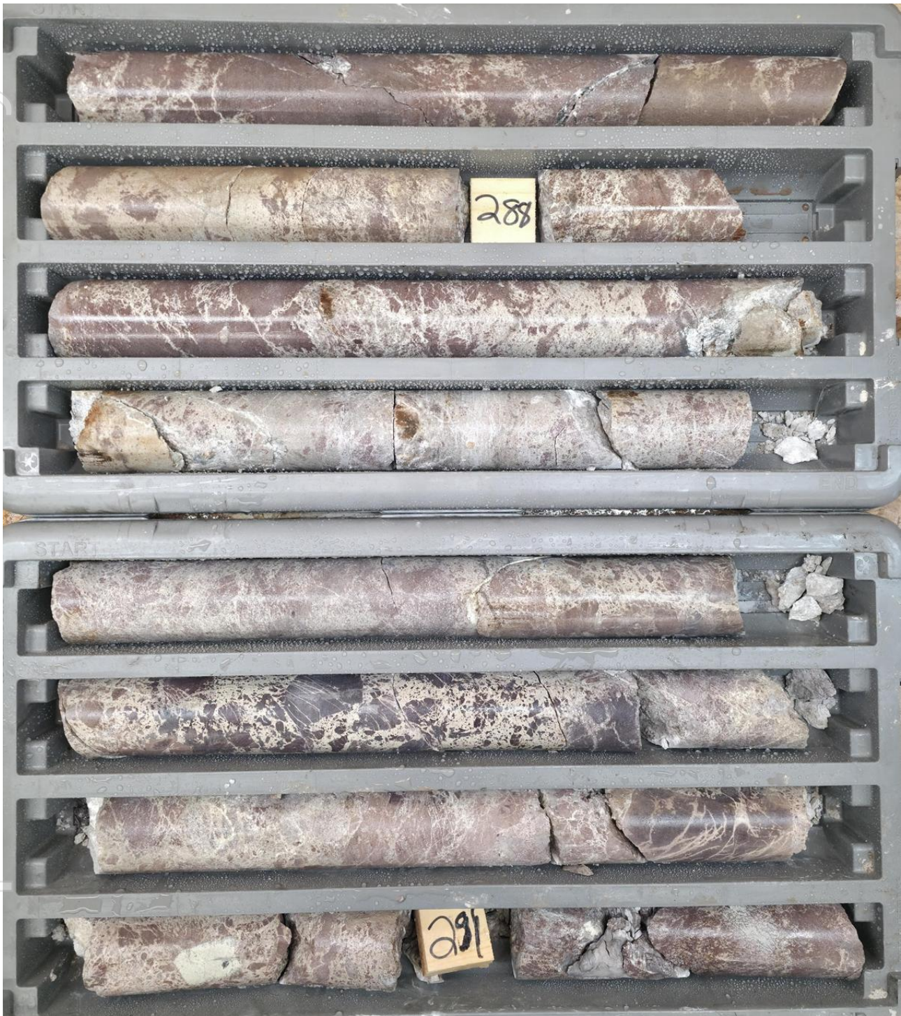
Figure 4. Drill core from DDCO26-001 showing the deeper hydrothermal breccia (288-291m depth) — interpreted to be the blind HSAMT conductor. Visual observations only; not a proxy for grade.
