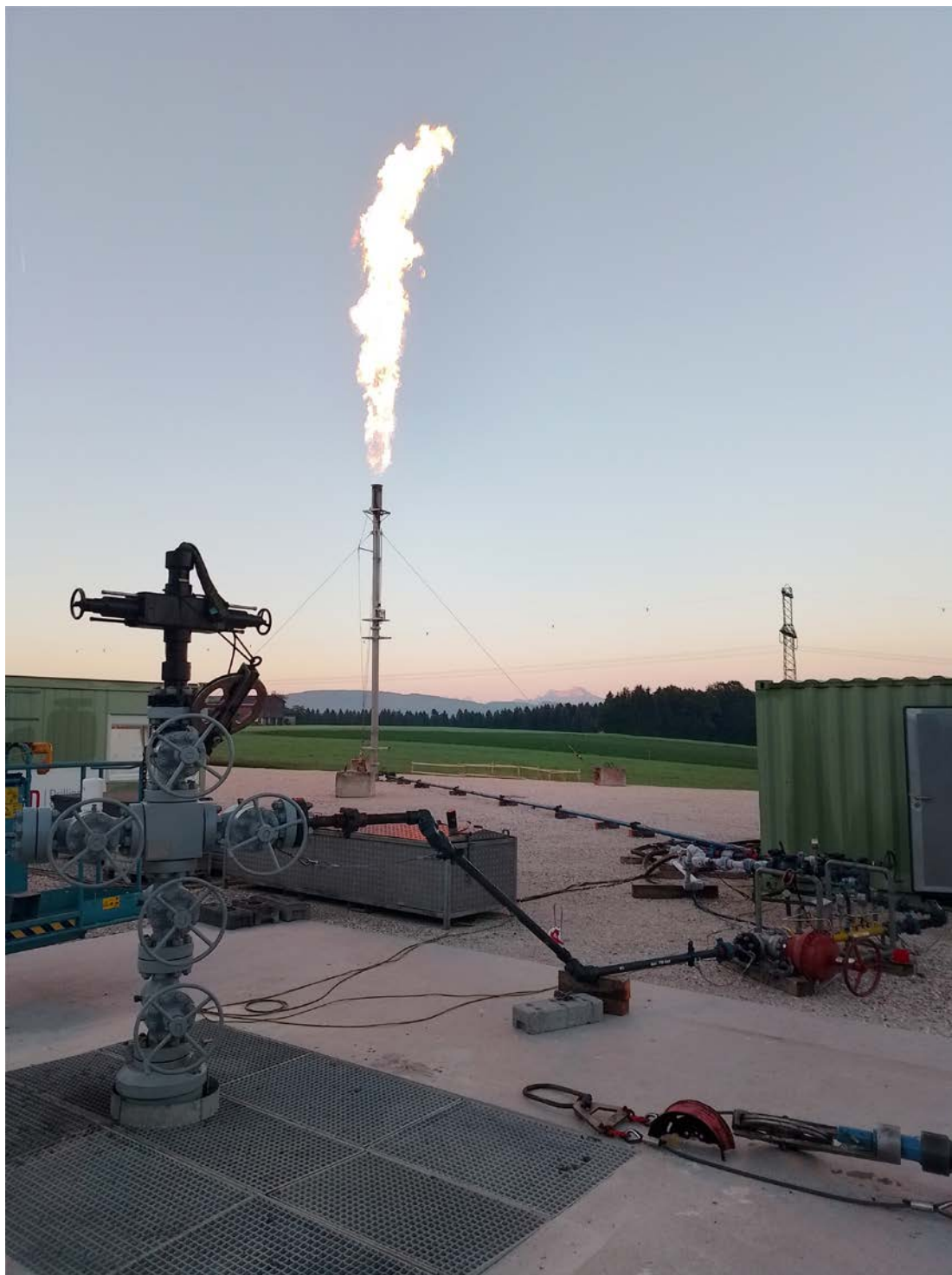
Zone 1 testing of the HOCH-1 shallow gas well in Upper Austria
