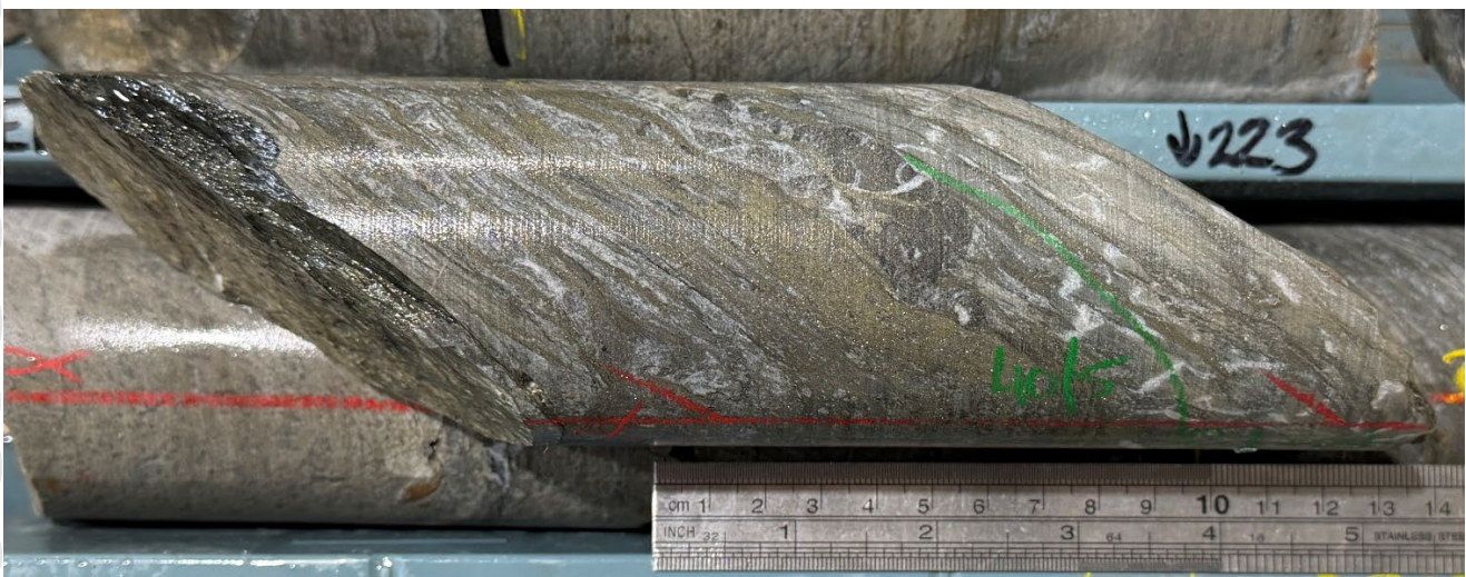
Figure 4: 25cm Section of uncut core, sheared, altered and mineralised from 223-224m in AEIDD001, the bright brassy coloured mineral is pyrite, a common sulphide mineral often associated with gold-bearing alteration systems.
