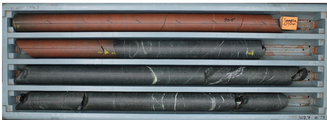
Figure 7. HDD26-01 logged aplite (reddish orange) indicating proximal felsic intrusion a potential driver of mineralised fluids.
