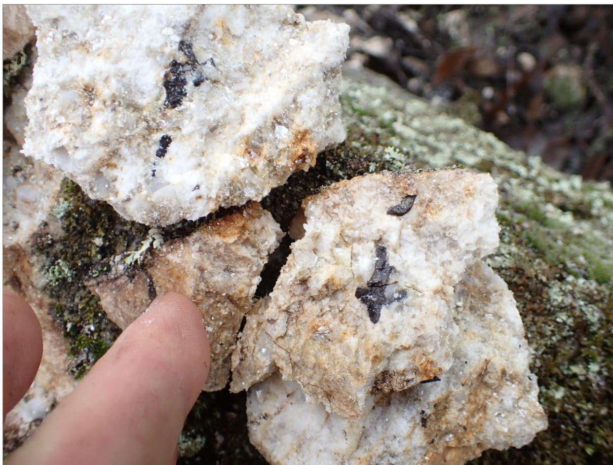
Figure 2 – Sample WWP001 1 showing interpreted black cassiterite in pegmatite boulder from the floor of the historic Walwa open pit
