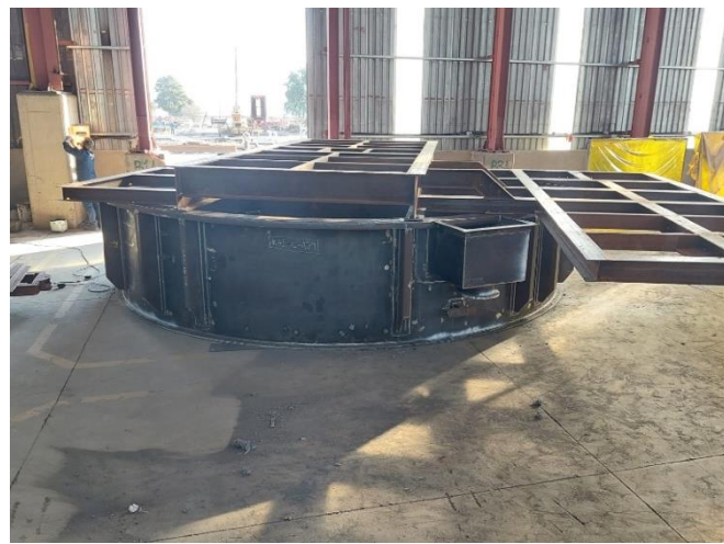
Figure 7: CIL Tank fabrication
